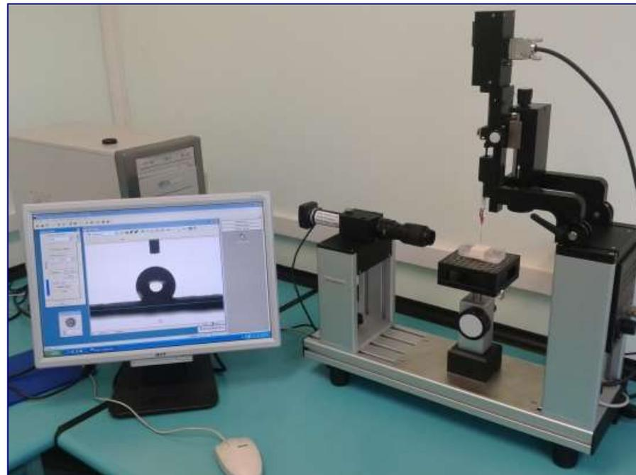
**Figure 4:** Optical Tensiometer
